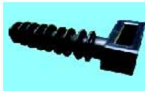
Designed with an additional push mount head these cable ties secure cable looms to a panel or chassis without the need of any other fixing device. The cable tie is fixed by pushing it into a panel of 2.3 mm thickness. Tensioning wings on the side of the head provide extra stability and overcome thickness variations in the
