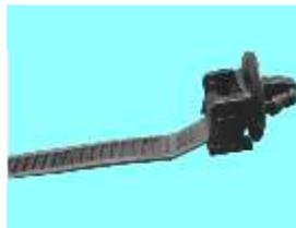
Novoflex Dome Fir Tree Mount Cable Tie can securely fix cable bunches to a panel or chassis, without the need of any fixing tool. This can be done by simply pushing the anchor through a plate with 0.6 mm – 2.6 mm Thickness and then tying the cables with the tie. The anchor fits perfectly into the hole of your chassis, providing a solid, rattle-free installation.
