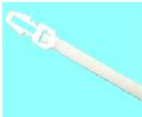
Designed with an additional Push Mount Head, these Cable Ties secure cable bunches to a panel or chassis without the need of any fixing tool. This can be done by simply pushing the anchor through a plate with 0.6 mm – 3.0 mm Thickness and then tying the cables with the tie. The small Stability-Projections just below the anchor, grip into the hole of your chassis by tightening the gap, thereby ensuring a very secure installation.
