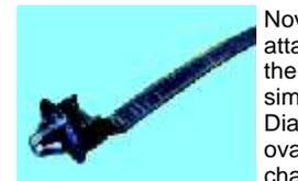
Novoflex Oval Push Mount Cable Tie can securely attach cable bunches to a panel or chassis, without the need of any fixing tool. This can be done by simply pushing the anchor through a 7 x 12 mm oval Dia Hole and then tying the cables with the tie. The oval anchor fits perfectly into the hole of your chassis, providing a solid, rattle-free installation.
